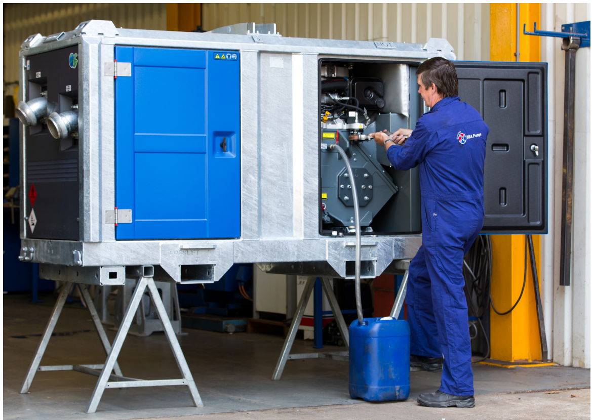
With the DriveOn® feature only 20 oil changes are required during an engine lifetime an estimated (30.000 hours).
