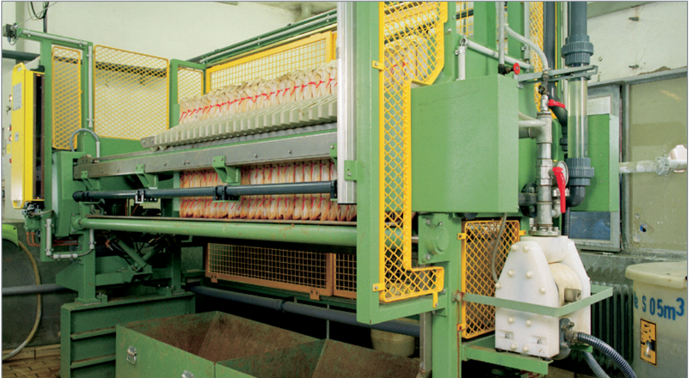
Fig 1: A typical chamber filter press being fed by a high-pressure air-operated double-diaphragm (AODD) pump (Almatec® AHD Series).
