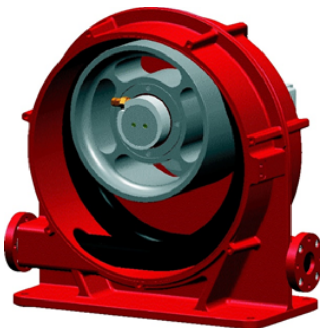
Figure 4. Depicts a Flowrox single roller design peristaltic pump. This design compresses the hose only once per revolution. Shoe design and double roller designs compress the hose two times per revolution. For this reason, the Flowrox pump hoses last minimally twice as long because they have one half the number of compressions. Also, since no heat is generated by the Flowrox design the hoses typically last 3 - 5 times longer than shoe designs.
