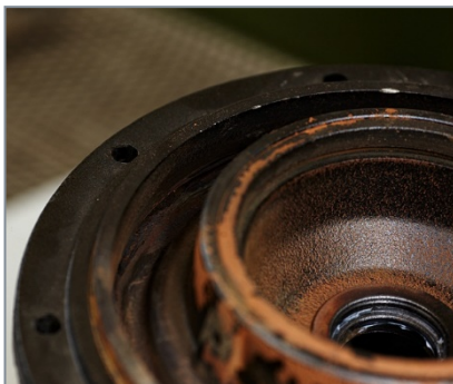
Disassembled corroded housing
