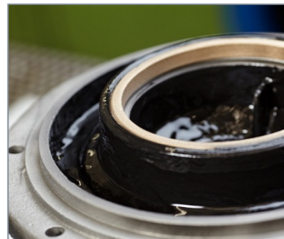
Protected housing before reassembly
