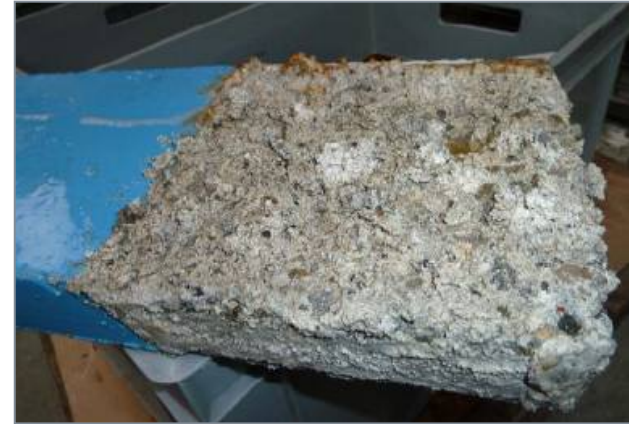
Chemical attack on concrete, protected vs. unprotected
