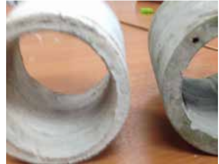
Abrasive wear on Teflon® bearings
