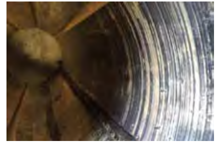
Abrasive wear on metal, select a grade with a higher hardness rating.
