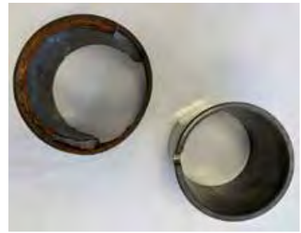
Cracking of carbon bearings
